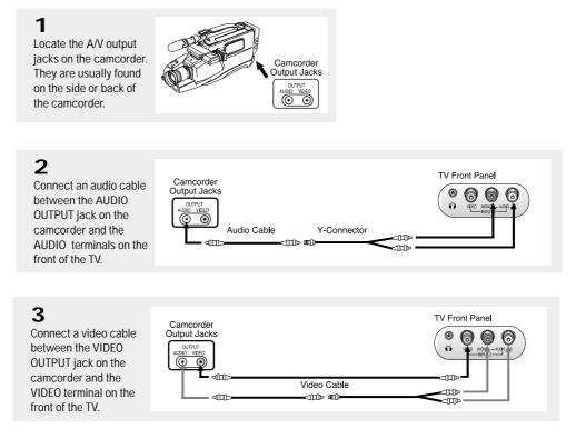
The audio-video cables shown here are usually included with a Camcorder. (If not, check your local electronics store.) If your camcorder is stereo, you need to connect a set of two cables.
